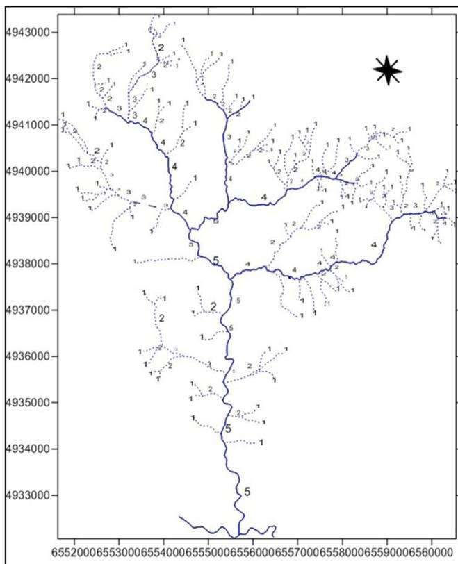
**Fig. 3. Ranking of the tributaries in the Solina drainage area according to Strahler**
